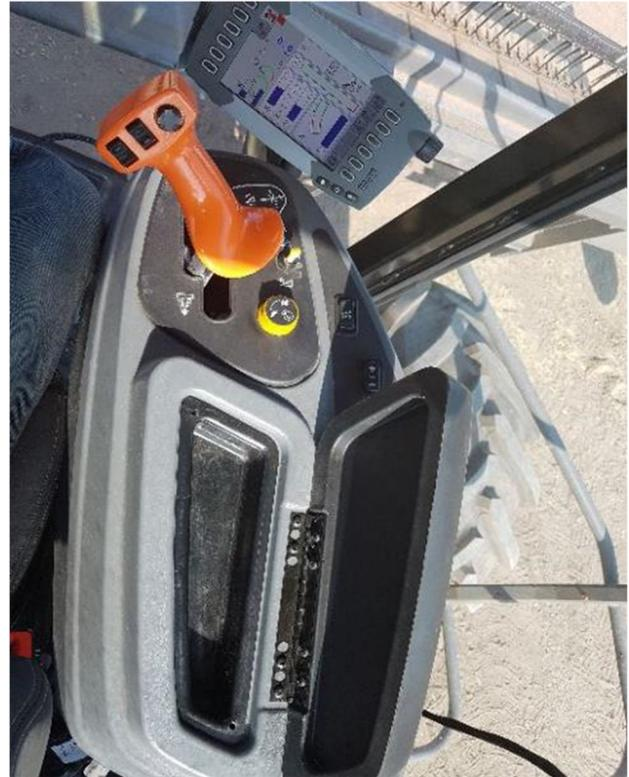
Inside the armrest you will find two 3-pin Deustch connectors plugged into their terminators. Remove both 3-pin Deustch plugs from their terminators. The Agra-GPS adapter cable will have two 'in-between' style connector pairs. The first connector pair (the pair that is under the same sleeving as the switched power/power/ground) is connected between the CAN 0 line, and a terminator. The other two plugs will be connected between CAN 1, and a terminator.
