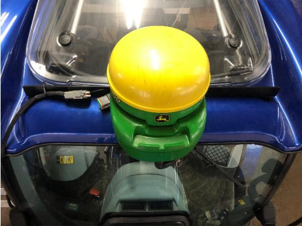
Also run the display portion of the long cable to a John Deere display (here a 4640).
