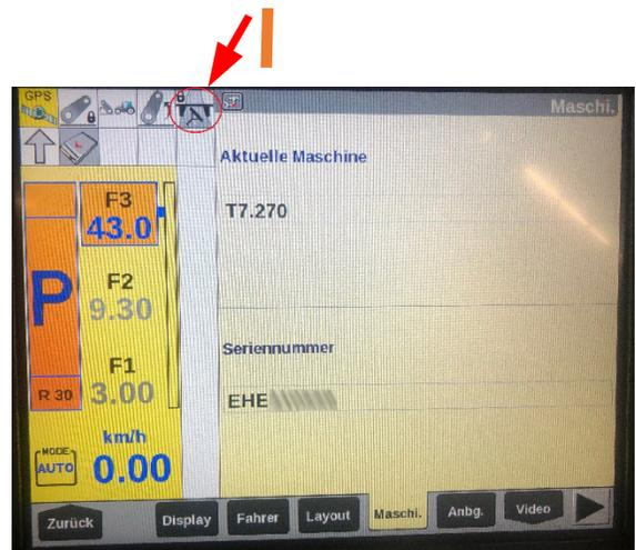
If you have a newer machine then 2017 make sure that the tractor is configured to ISO BUS Steering. It's the same configuration like using a Trimble XCN-1050™ Display.
