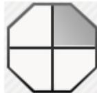
Tractor controller is performing self-checks/ not ready to accept commands.
