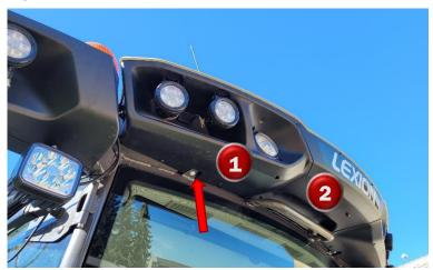
Install with bracket <u>square</u> to machine and flush to the front of the eyebrow. Drill through plastic and install bolts with locking nuts.
