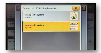
On John Deere 1800, 2600, 2630 the application will be shown in the side menu of the John Deere display. The side menu is opened by clicking the button on the bottom right of the display.
