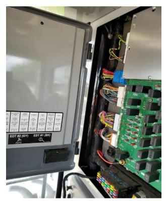
Use the two diagnostic port connections to connect to the Gleaner JD-Bridge. Both of these diagnostic ports are visually the same, so care is needed to make sure the proper connections are made. The main diagnostic port of the Gleaner-JD Bridge (labelled Main) is connected to the rightmost diagnostic port, while the secondary diagnostic port of the Gleaner-JD Bridge (labelled Secondary, and contains only 1 green and 1 yellow wire) is connected to the leftmost diagnostic port.
