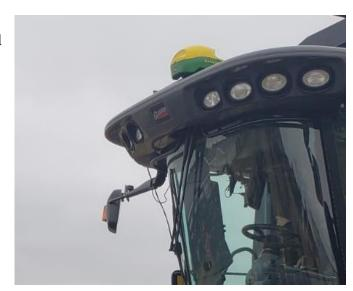
Use the provided adapter cable to connect the 12-pin deutsch of the JD GPS receiver with the 12-pin deutsch of the Gleaner-JD cable.
