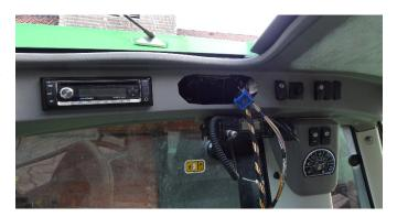
Find the blue 15-pin connector XC10 and open the connection. The connector is located to the right of the opening. Insert the Agra-GPS adapter harness into the 2 \* 15-pin connection points and place the Deutz-JD Bridge in the opening to the right.
