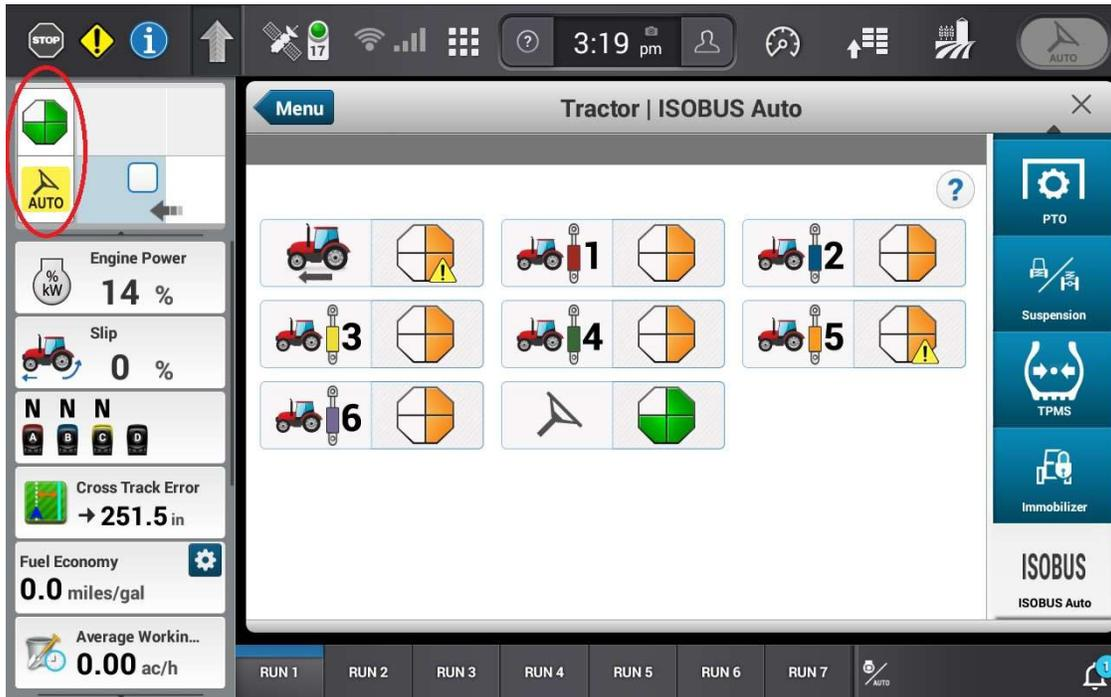
In the picture above, the external guidance system is ready to steer the tractor. The operator just needs to press the Auto button on the joystick.
