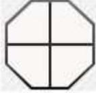
ISOBus Class 3 is off. This means the tractor controller has not initialized or the system has been cancelled.
