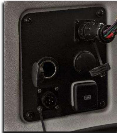
The next connector will be installed into a diagnostic port located under the passenger seat of the machine.
