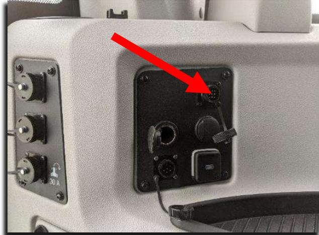
Connect the smaller 9-pin female connector of the Agra-GPS bridge to machine adapter into the 9-pin male ISO connector of the machine.
