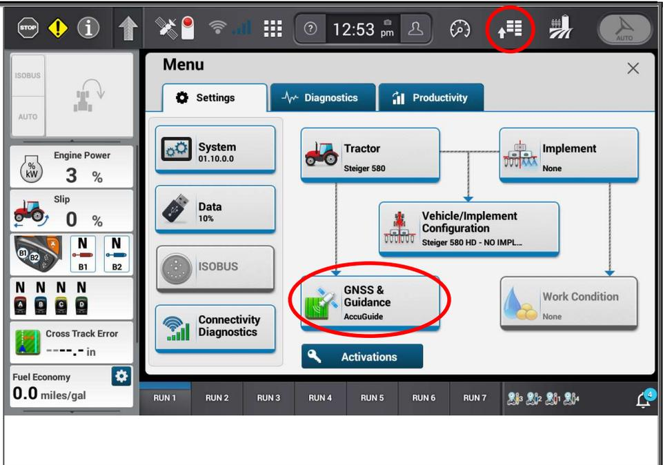
2. Ensure Vehicle Receiver is set to "Not Installed"
