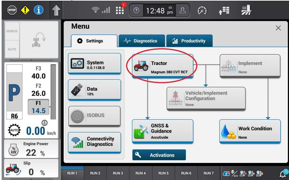
c. Scroll down on the right side to the steering page and check to make sure the steering mode is in off-road mode. The tractor must be in off road mode for external guidance to work.
