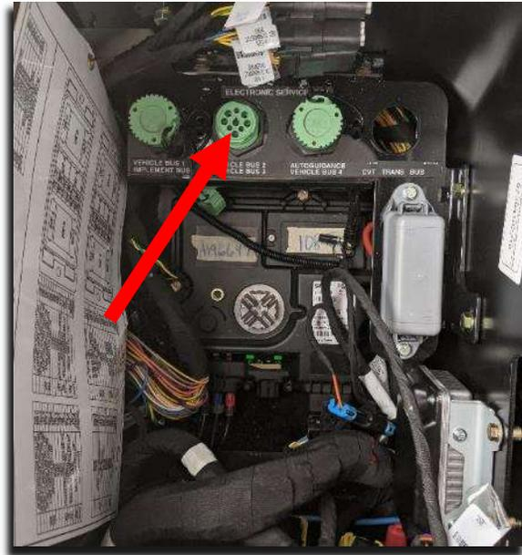
Insert the larger 9-pin female connector of the Agra-GPS bridge to machine adapter into the middle 9-pin male diagnostic port labelled, 'VEHICLE BUS 2' 'VEHICLE BUS 3'
