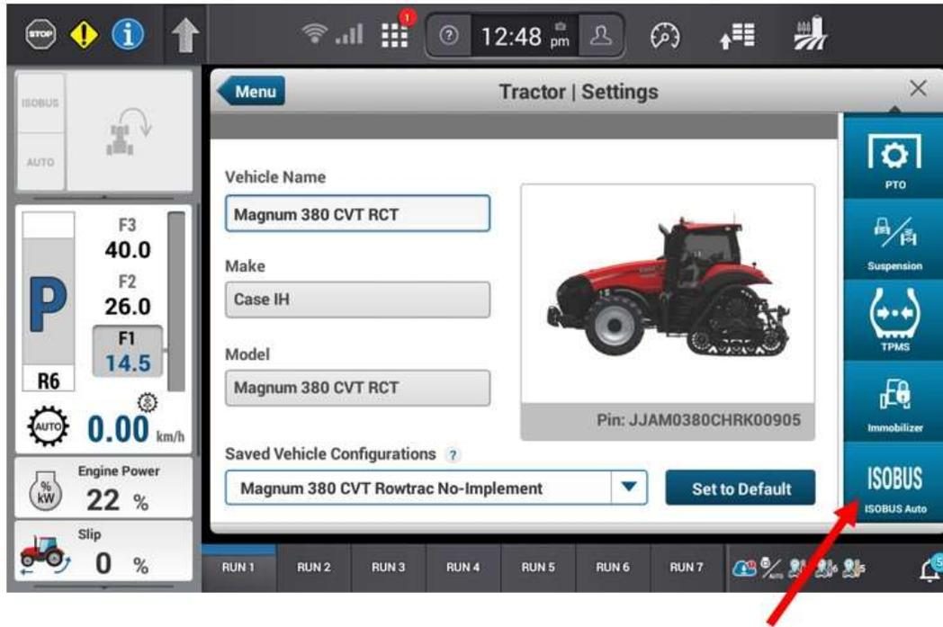
f. Depending on what ISOBus Class 3 activations the tractor has, this page may have different icons on it. For external guidance, look for the icon with the steering wheel, as shown below. (If the icon is not present, the tractor does not have ISOBus Class 3 activated. It will have to be activated by a CNH dealer.)
